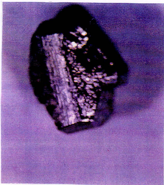
Fig.III.33:- - Equant grain of pyrite with triple junction and straight boundaries.
