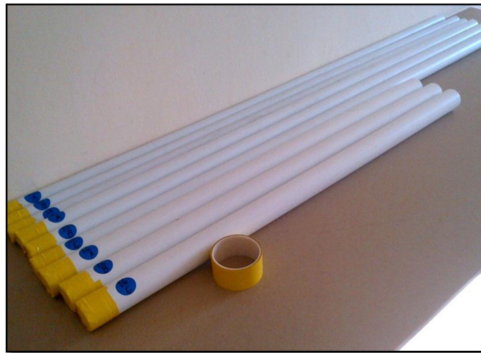
Figure 31, 27.8mm, 36mm and 45mm ID PVC pipes prepared for VOD Test 3
