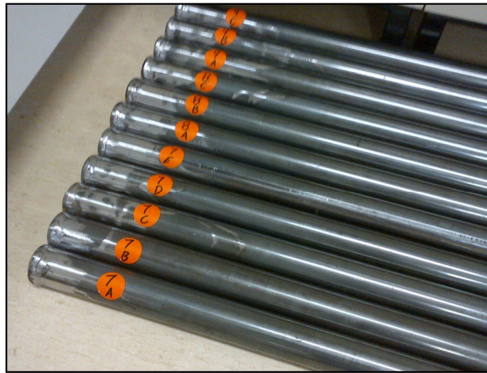
Figure 28, Steel pipes with a single end welded closed prepared for VOD Test 4
