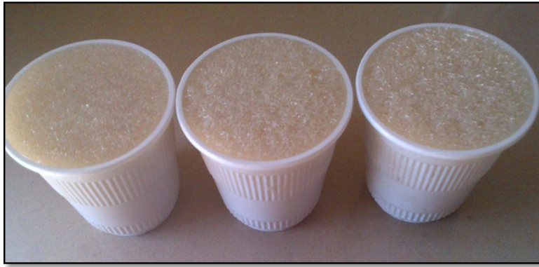
Figure 23, Sequence of three Emulsion B samples taken to establish gassing rate under controlled conditions.
