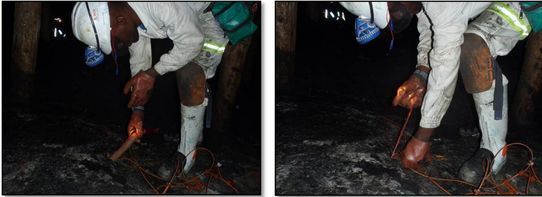
Figure 37, Sequence of photos showing operator inserting a Vala stemming plug while loading a winch bed
