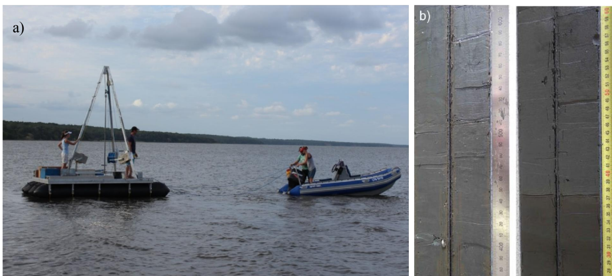
Figure 4.2: a) Barge and piston coring system used to extract sediment cores and b) inset of the dominantly clay rich core sediments.
