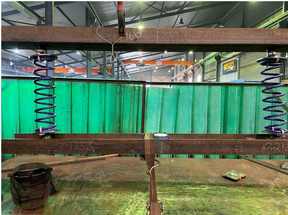
Figure 162: Experimental setup to impose initial conditions on the springs
