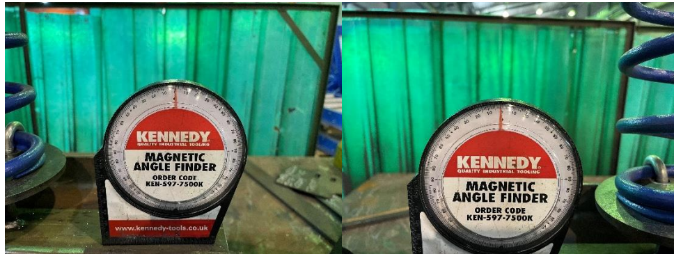
Figure 163: Angle finder results on each end of the rigid bar presenting a 0 inclination
