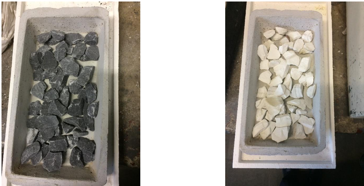
Figure 4.41: Sample Z before (left) and after calcination (right) at 1050 °C for 1 hour.
