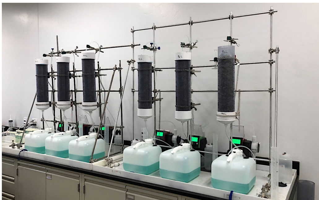
Figure 13: Column setup to test effect of leaching aid on acid consumption. BASF Laboratory, Tucson, USA.
