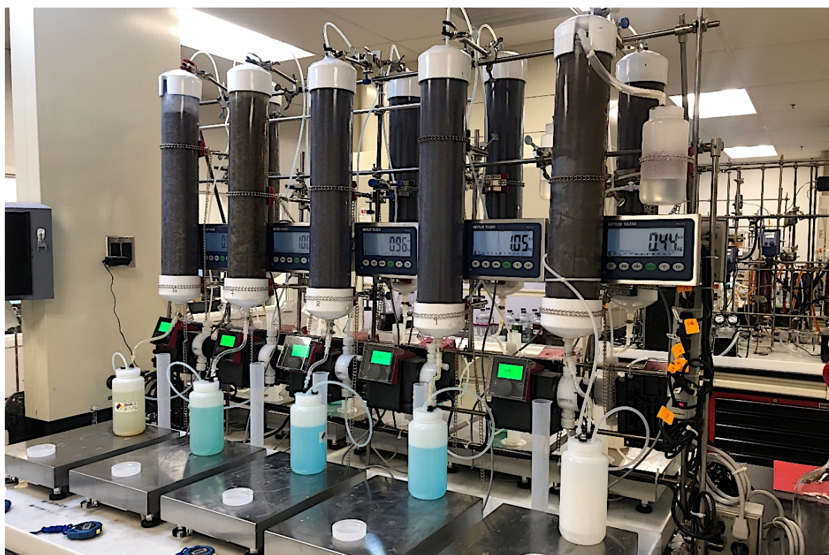
Figure 10: Column setup to investigate effect of leaching aid on solution drainage. BASF Laboratory, Tucson, USA.
