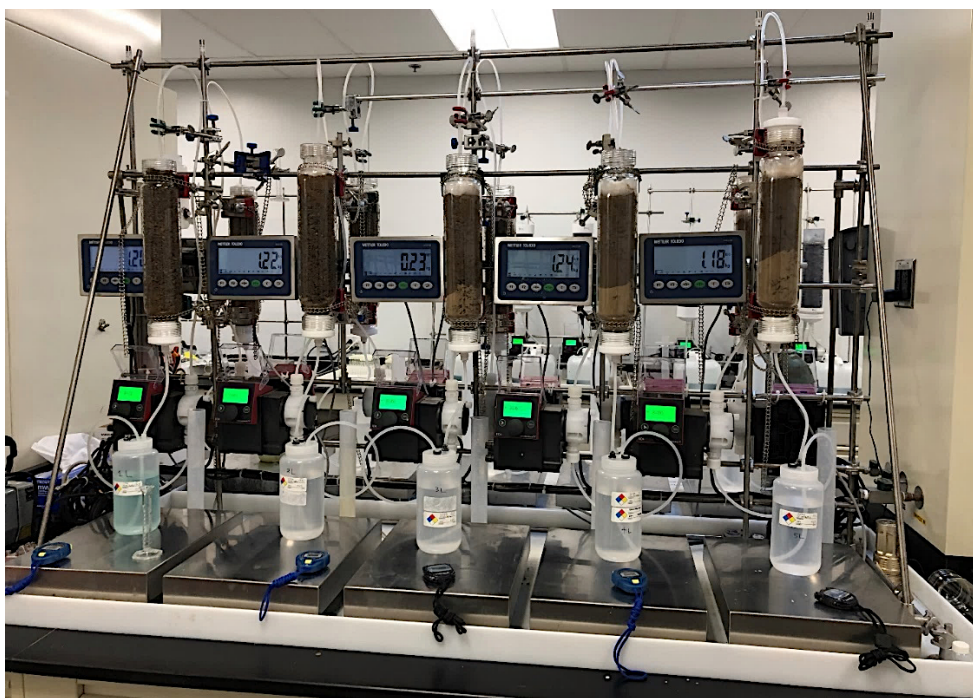
Figure 12: Column setup to test effect of LixTRA on flow through different particle size distributions. BASF Laboratory, Tucson, USA.
