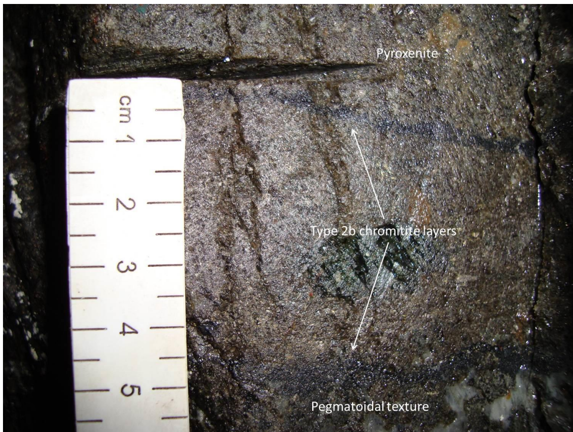
Figure 2.4.2: Photograph showing a close up of the Type 2a chromitite layers from the Thin facies. An underground sample was cut from this portion at 23 level, K3 Vertical Shaft.
