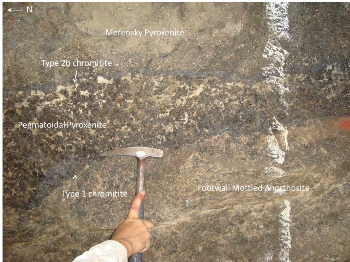
Figure 2.4.5: Photograph showing the thinning of the RPM facies and transgression of the Type 1 chromitite layer into the footwall anorthosite in an underground raiseline at 26 level, K4 Vertical Project Shaft.
