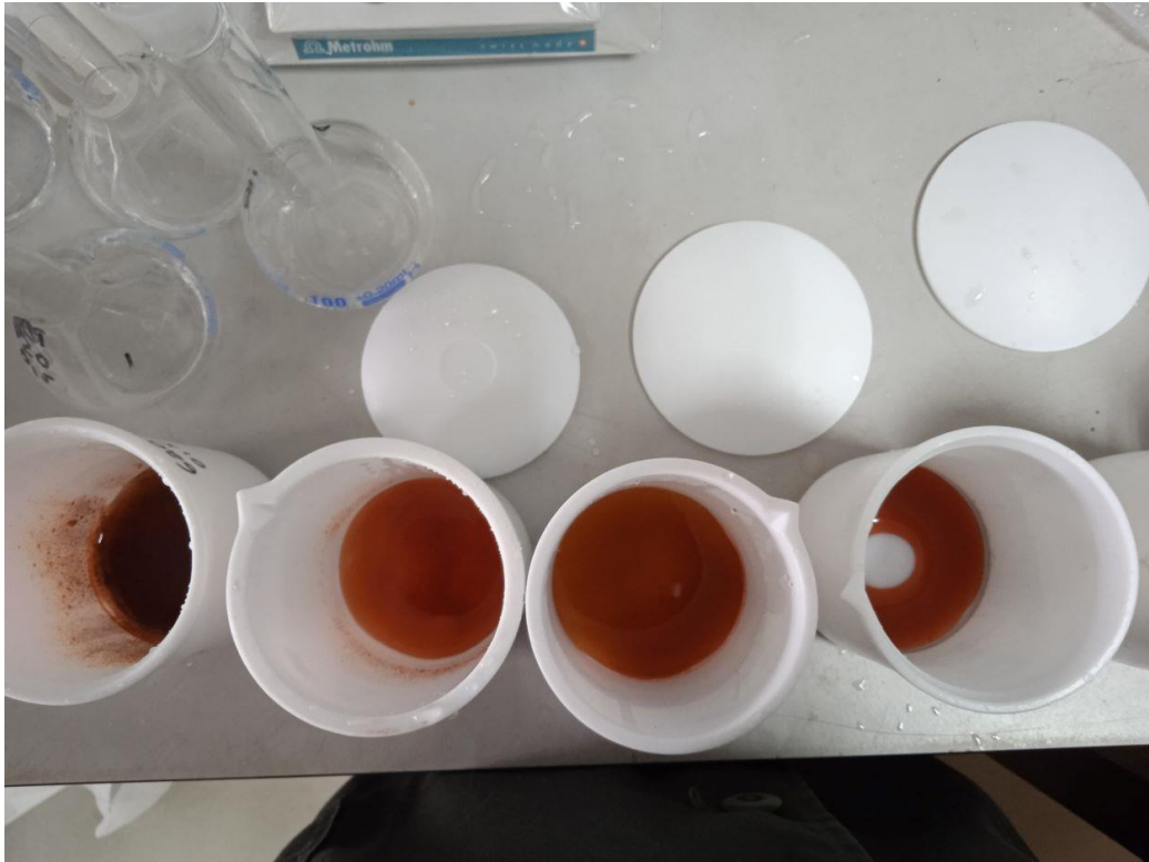
Figure 3.7. Teflon beakers with acid-digested samples
