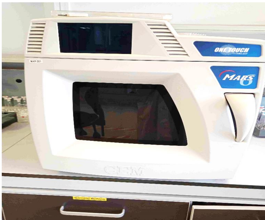
Figure 3.6. CEM Mars6 microwave digestion instrument
