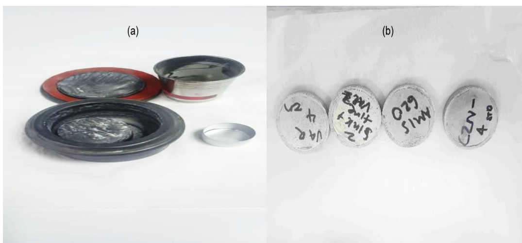
Figure 3.3. Tungsten carbide bowl used for sample preparation (a) and the obtained pressed pellets (b).
