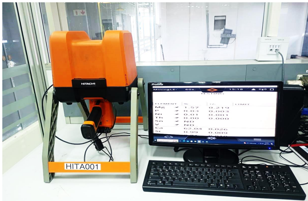
Figure 3.2. Hitachi X-met8000 used for elemental composition
