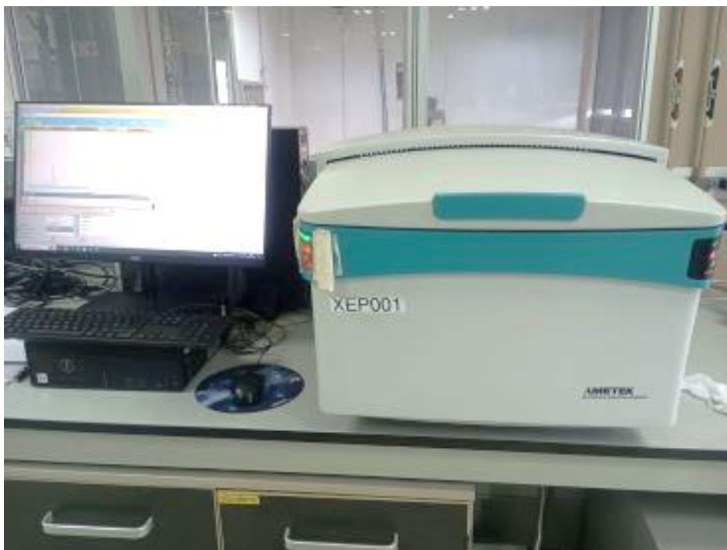
Figure 3.4. Xepos He EDXRF was utilised in the analysis of the pressed pellets
