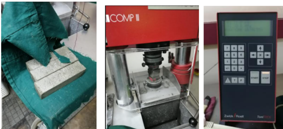
Figure 16. Specimens in damp cloth, crushed to get Compressive strength in MPa (left to right)
