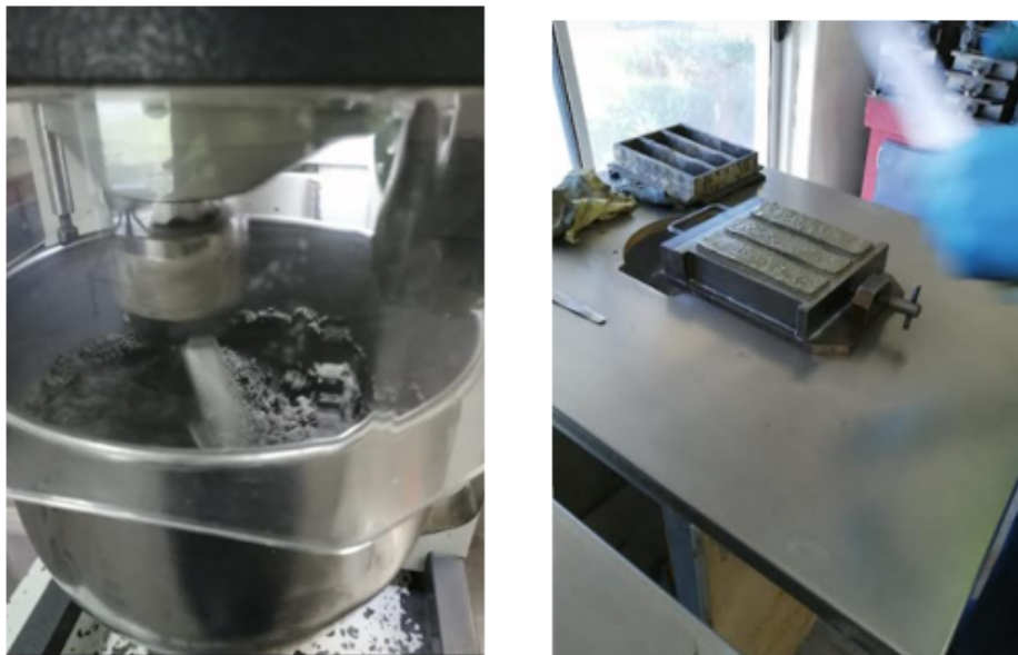
Figure 13. mixing bowl in action(left) and mold filled with paste (right)
