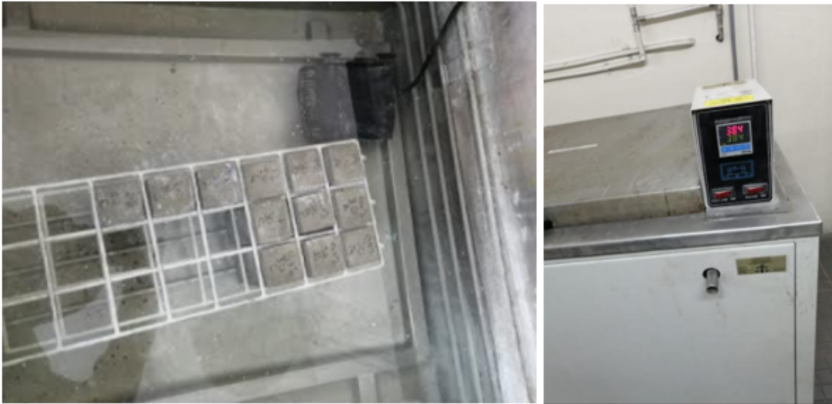
Figure 15. specimens cured in water(left) inside 38 degrees container(right)
