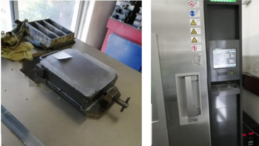
Figure 14. mold covered and labeled(left), controlled cabinet (right)
