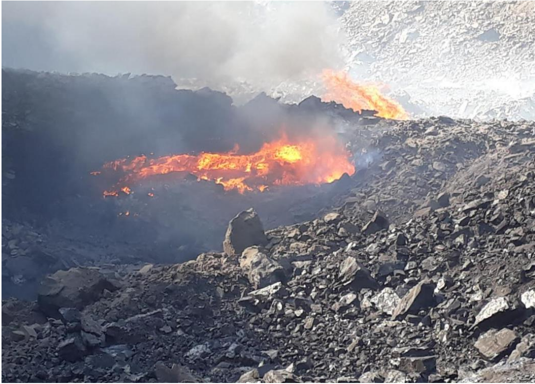
Figure 8.1: Khwezela Colliery spontaneous combustion
