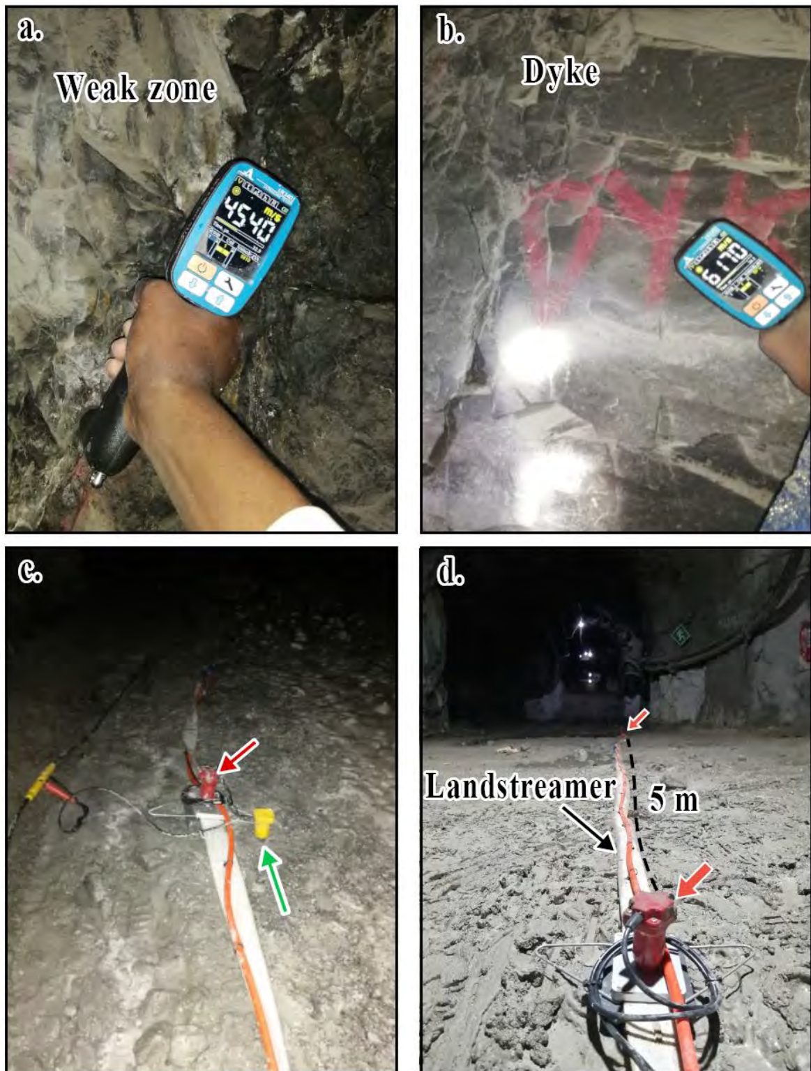
Figure 4: Measurements of the seismic velocities underground using ultrasonic pulse meter over a) a weak zone and b) a dyke. The set-up inside the tunnel of the seismic survey using the seismic land streamer (red arrows) and planned geophone (green arrows) is shown in c) and d)
