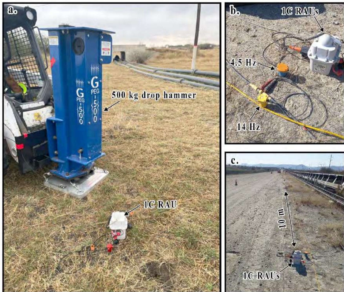
Figure 6: Seismic source and receivers used during the Maseve surface seismic acquisition (August 2022). a) Photo of the G-PEG 500 drop hammer, and b) Sercel UNITE wireless 1C
