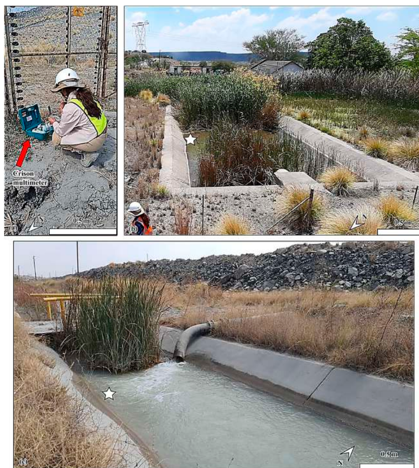
Figure 4. (a) An example of how the field sampling was carried out in the study area using the Crison Multimeter. (b) Tailings Storage Facility 1 (TSF 1) sample location (indicated by the white star). (c) Tailings Storage Facility 2 (TSF 2) sample location (indicated by the white star).
