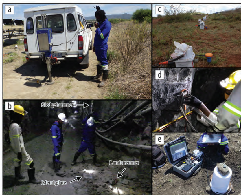
Figure 4. Seismic sources and the different receivers that were used during the Maseve mine acquisition (November 2020). (a) A 48 kg accelerated weight drop mounted on a vehicle along remote acquisition units. (b) Data acquisition in the mine tunnels using a sledgehammer as a source and 4.5 Hz receiver landstreamer. (c) Sercel Unite wireless 1C receivers used for passive seismic studies. (d) Underground mounting of the 4.5 Hz receiver landstreamer on the sidewall supported by roof bolts. (e) Photo of a broadband seismometer buried in the ground to record mine induced events.
