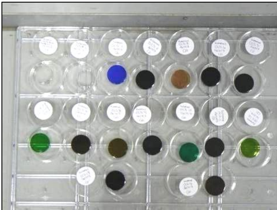
Figure 5-5: Calibration standards prepared with the Katanax and potassium iodide as the non-wetting agent
