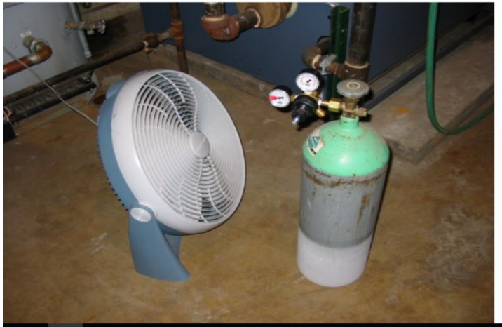
Figure 3.3 Fan and CO 2 gas tank connected to a gas regulator. Source: Escombe et al., (2007).
