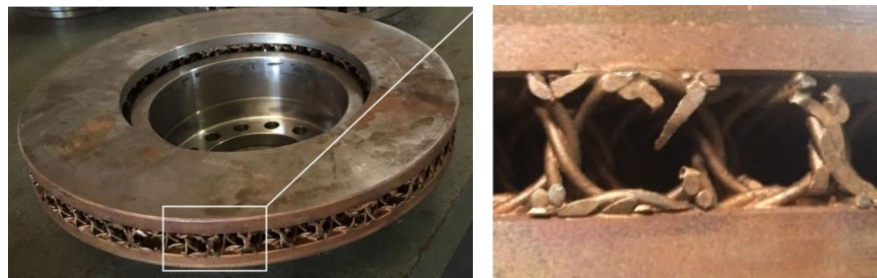
Figure 1.6 Custom made brake disc with Wire-woven bulk diamond (WBD) core used in the ventilated channel
