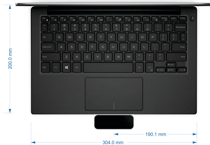
Figure 2.2.1: Top view configuration of the Leap Motion with the laptop.
