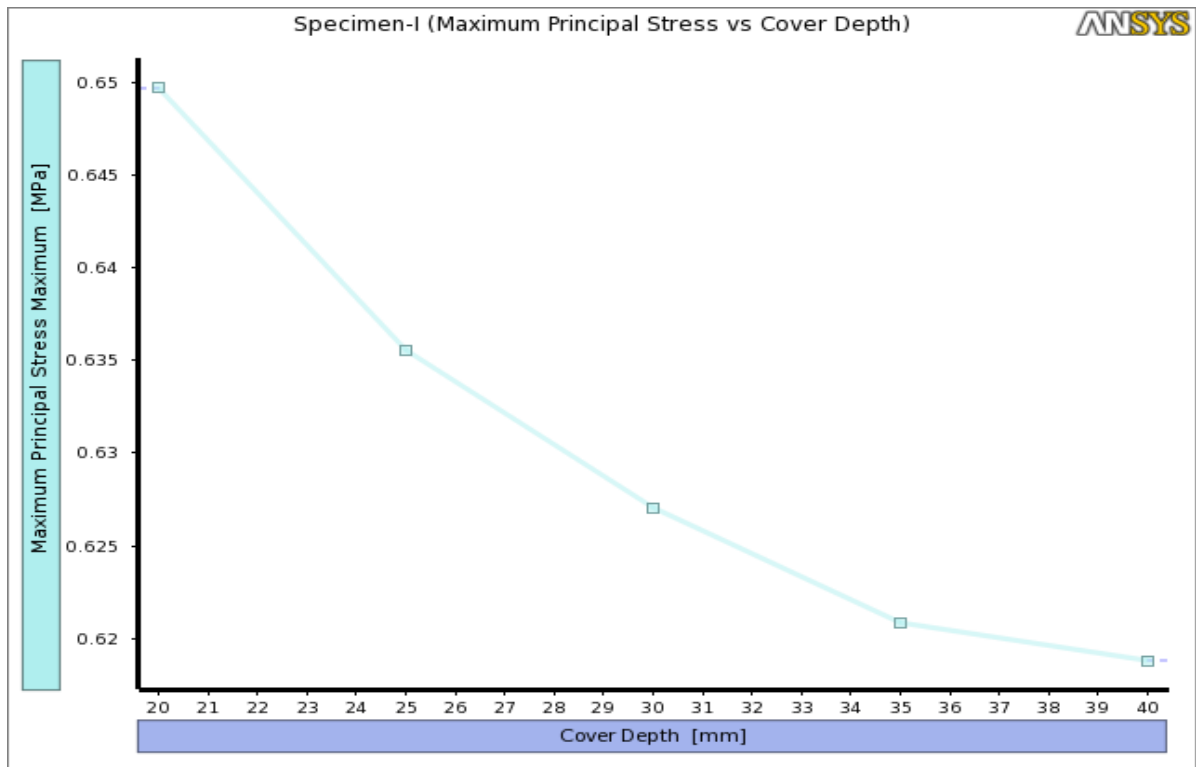
Figure 6. 11 Maximum Principal Stress vs Cover Depth (Case II, SP-I)
