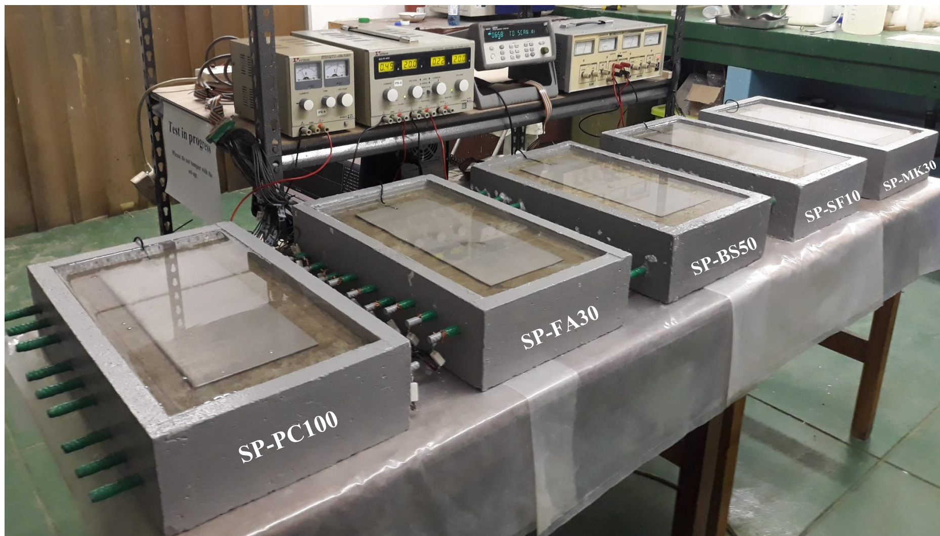
Figure 3. 16 Setup of the Impressed Current
