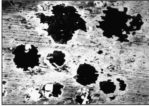
Figure 2- 7 Micrograph (350x) of 304L stainless steel exposed to 2.5 M sodium chloride at +400 mV vs SCE for 10 minutes (Ibrahim et al. 2009).
