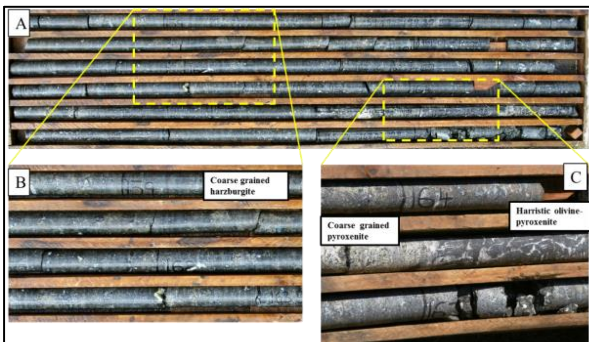
Fig. 3.4. Diamond drilled core from (A). 158.7 to 163.52m. (B) Typical coarse grained harzburgites. (C) Coarse feldspathic pyroxenite in contact with harzburgite-textured olivine-pyroxenite.
