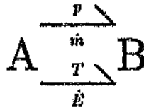
Figure 3.12: The double bond found in pseudo bond graphs of compressible thermofluid systems.
