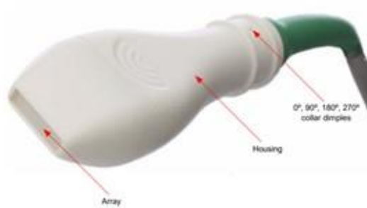
Figure 5.2: Probe used by the Vevo ® 2100 in viewing the rabbit eyes. This probe allowed for the viewing of the rabbit eyes through ultrasound techniques
