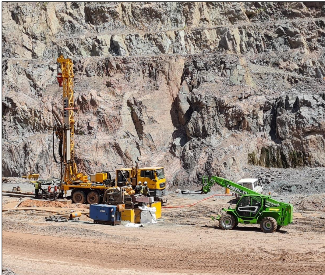
Figure 35 - RD drilling process (Sociedade Mineira de Kaixepa Geology Department, 2024)
