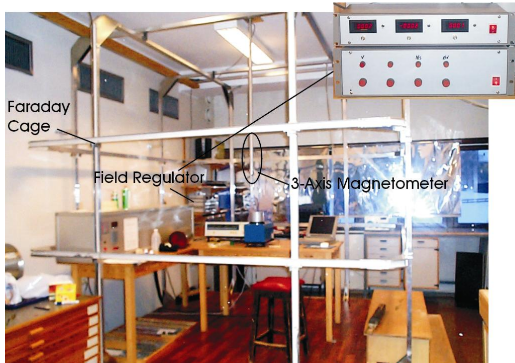
Figure 2.21 Faraday cage, containing the spinner magnetometer and thermal demagnetiser. The field is monitored with the use of a 3-axis magnetometer and is then automatically compensated for any change in magnetic field with the use of a field regulator, (insert top right).
