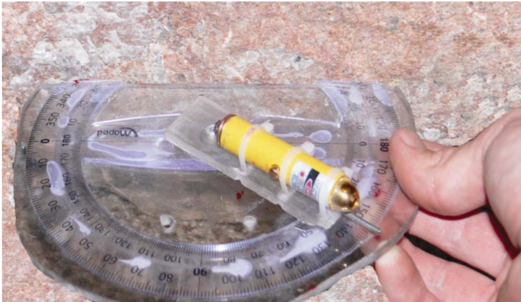
Figure 4.33 Orientation device used to accurately orientate samples underground. The flat end of the device is placed along the strike of the rock and the laser pointer is then pointed towards the survey peg, where the bearing is read off.
