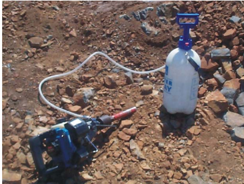
Figure 2.16 Portable gasoline-powered drill fitted with a non-magnetic diamond drill bit and water pump used to cool the drill bit during drilling.
