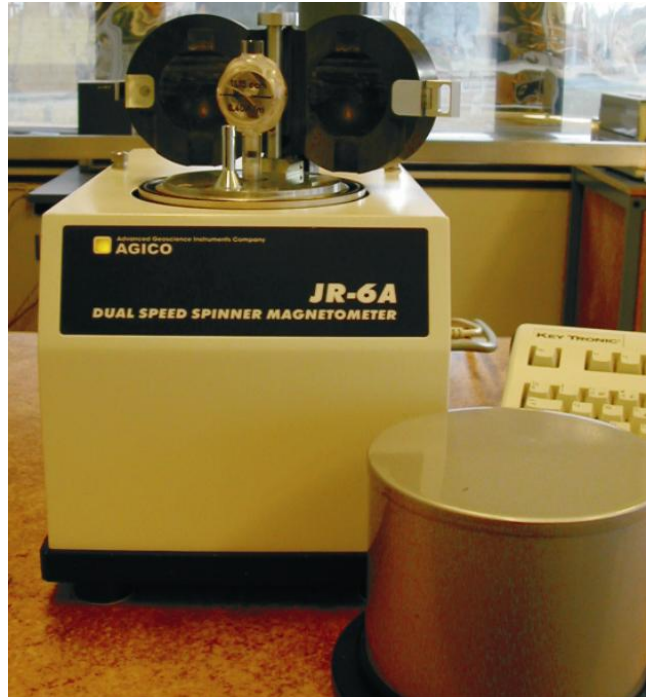
Figure 2.25 JR-6A spinner magnetometer, with \mu -metal shield removed to reveal pickup coils and sample holder and spinner system.
