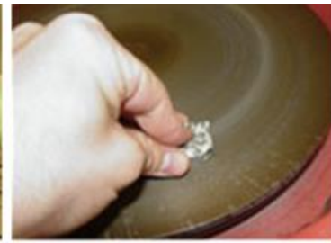
Step 3. Grinding the tablet to remove any saw or wire cutter marks
