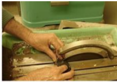
Step 2. Cutting rock to a tablet ~26 mm wide x 46 mm long x 5 mm thick.
