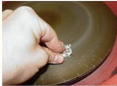
Step 5. Grinding top surface to a ~30 \mu\text{m} thickness, polishing to a 0.1 \mu\text{m} roughness.
