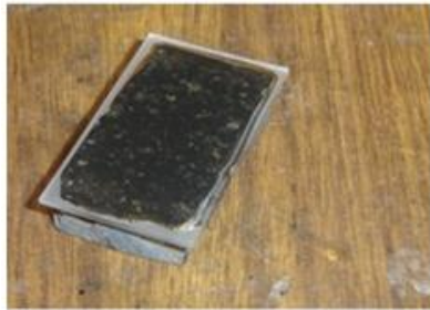
Step 4. Epoxy the rock tablet's ground surface to a glass slide
