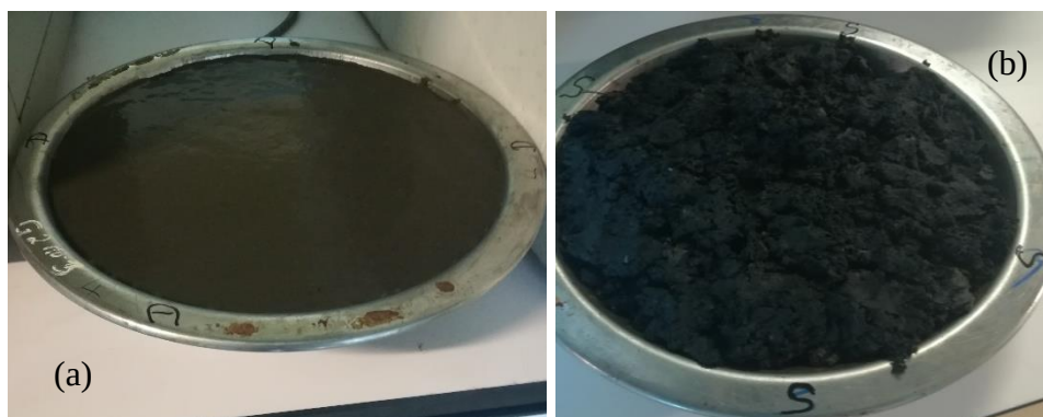
Figure 3.1 (a) Dissolved Air Flotation and (b) Final Sludge.
