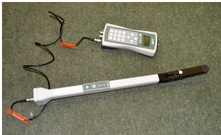
Figure 4.11: The LAI-2200 Plant Canopy Analyzer used to measure the average Leaf Area Index (LAI) for the riparian vegetation.
