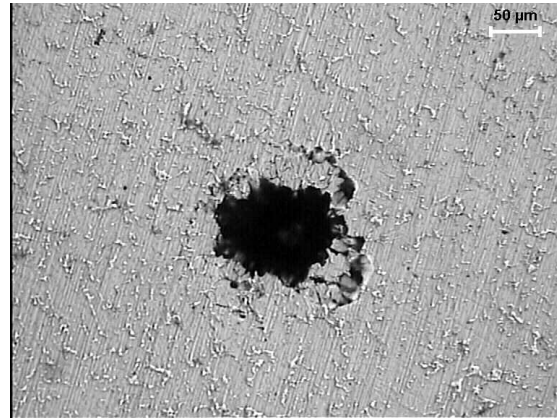
Pt 10 :Al 80 :Cr 10 Major interdendritic cracking
