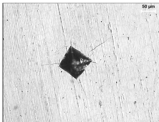
Pt 3 :Al 35 :Cr 62 Wavy slip and major cracking
