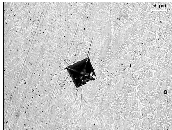
Pt 20 :Al 40 :Cr 40 Major cracking
