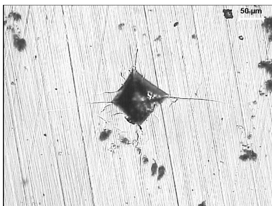
Pt 3 :Al 65 :Cr 32 Major cracking
