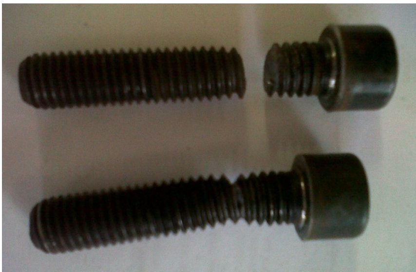
Figure 27: Sheared and snapped bolt from the pressure vessels/reactors
