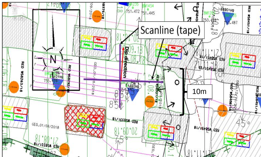
Figure 3.1: The Mine plan indicating mapped panel and the direction of the scanline tape.
