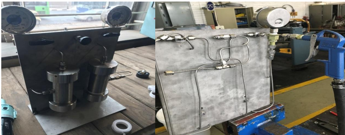
Photography 2: Air Separator Unit
