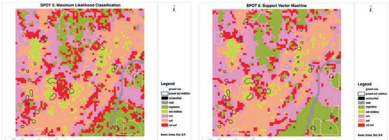
FIG. 6. (Left) BC2 for SPOT5 classified using MLC. (Right) BC2 for SPOT5 classified using SVM.
