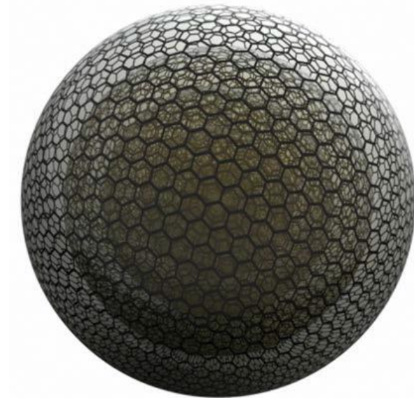
Scheme 9.1: The architectural structural model of CNO that exhibit multiple and concentric graphitic layers [19].
