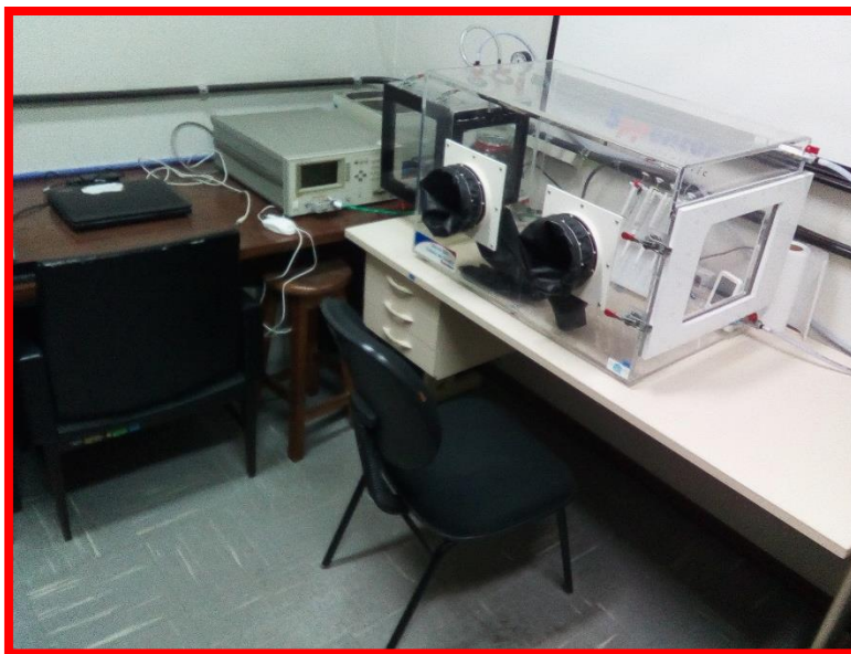
Figure S8.1: A photo that shows the LCR meter and glove box set-up used during the static characterization.
