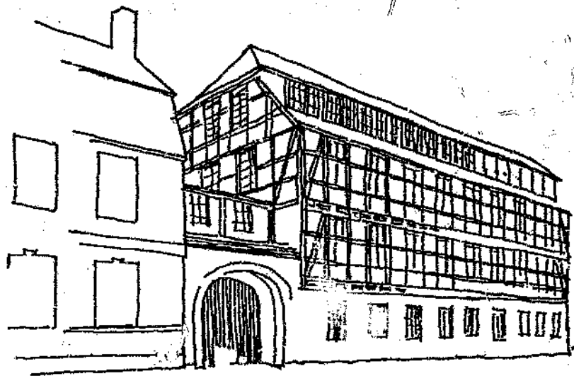
Fig.3 A textile factory built in 1756 at Luckenwalde in the district of Potsdam, Berlin which was famous for its cloth and hat factories. Note the set-back fourth floor with continuous window in the timber-framed building. It was a combination of ship-and-millwright construction common in many localities in Europe and Britain [Henn, Vol.1, 1955:21].
