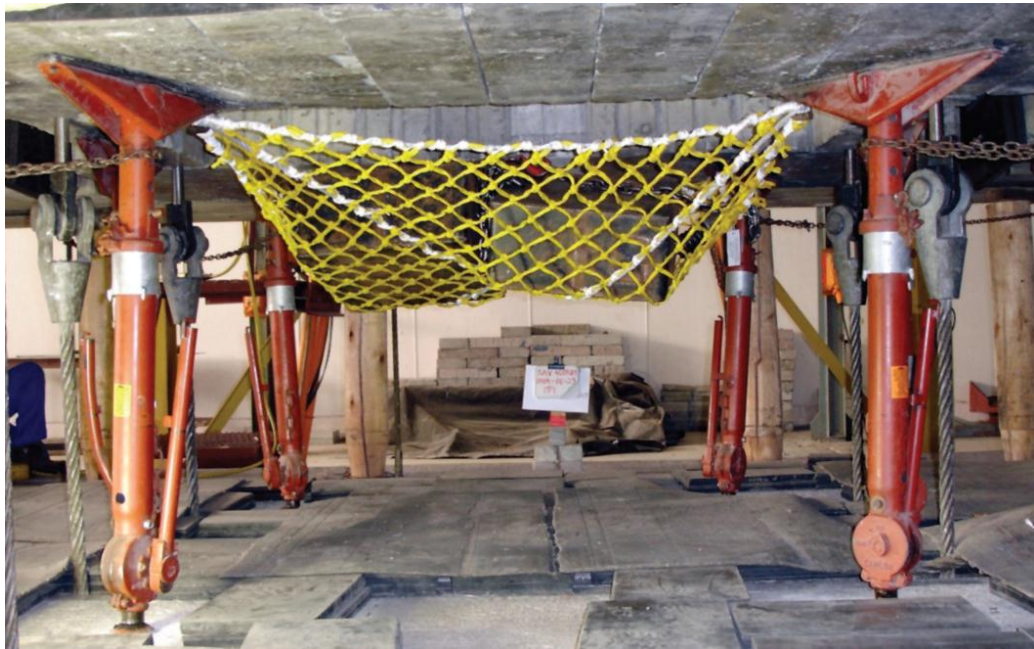
Figure 6.2.1 Safety net test at the Savuka testing facility. (Source: Skarbovig, 2010)
