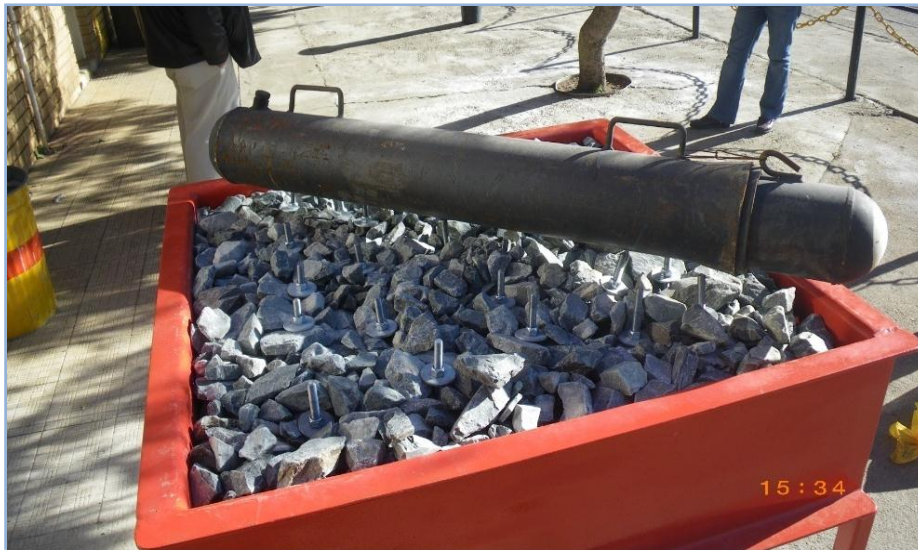
Figure 7.2.7 A rock prop is placed on top of the beam created demonstrating the strength of the beam created.
