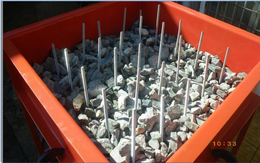
Figure 7.2.4 Broken rock between the bolts compressed. (Source: Gold Fields, 2012)
