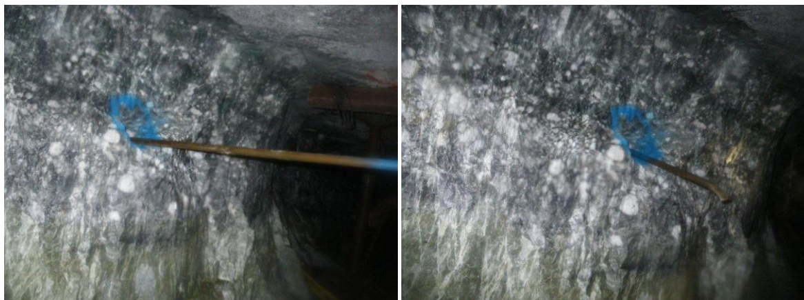
Figure 5.6.1 Checking of a Pre-conditioning hole at Thuthukani Shaft, KDC. (Source: Personal Collection)
