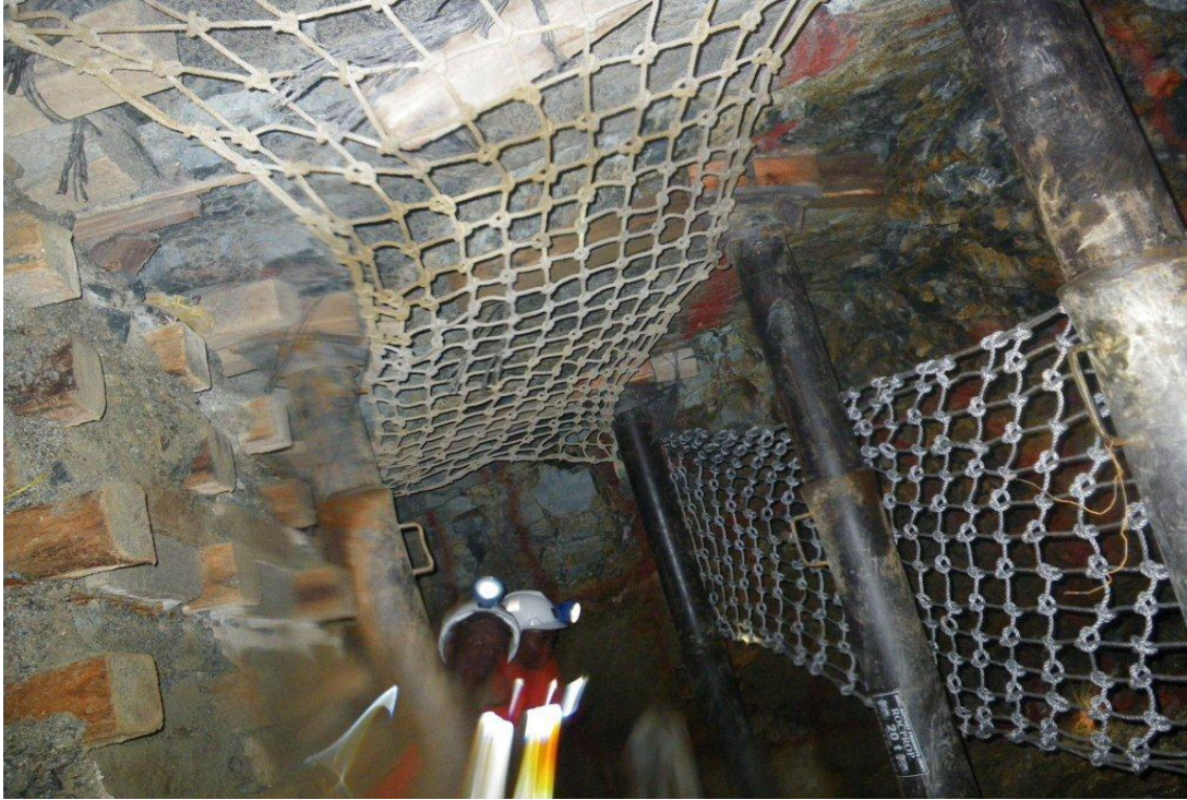
Figure 6.3.1 In-stope netting at Thuthukani Shaft, KDC.
