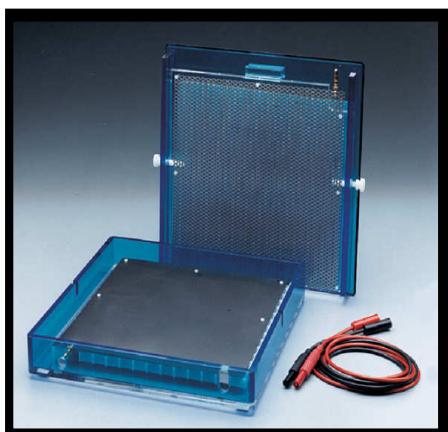
Figure A2.1: The semi-dry Electrophoretic Blotting System. The Sigma model B2529 is a plastic box (blotting chamber) inside which are contained two steel plates which act as electrodes, a stainless steel cathode and platinum coated anode. The blotting chamber is closed on top with a safety cover into which the power leads can be inserted. (SIGMA, St. Louis, MO). Photograph accessed on 1.8.2005, from the Web site: http://www.Sigmaaldrich.com/catalog/search/ProductDetail/SIGMA/B2529
