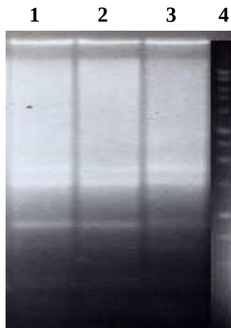
Figure 2.2: Agarose gel resolution of EcoRI digested DNA for the SH technique. Lanes 1: HuH7; 2: Hep3, 3: PLC/PRF/5; 4: (3 mm wide) 1 kb molecular weight marker (Promega). The DNA was evenly digested (A: lanes 3-6) and the same signature for the EcoRI RE is clearly visible for both the samples and the controls.
