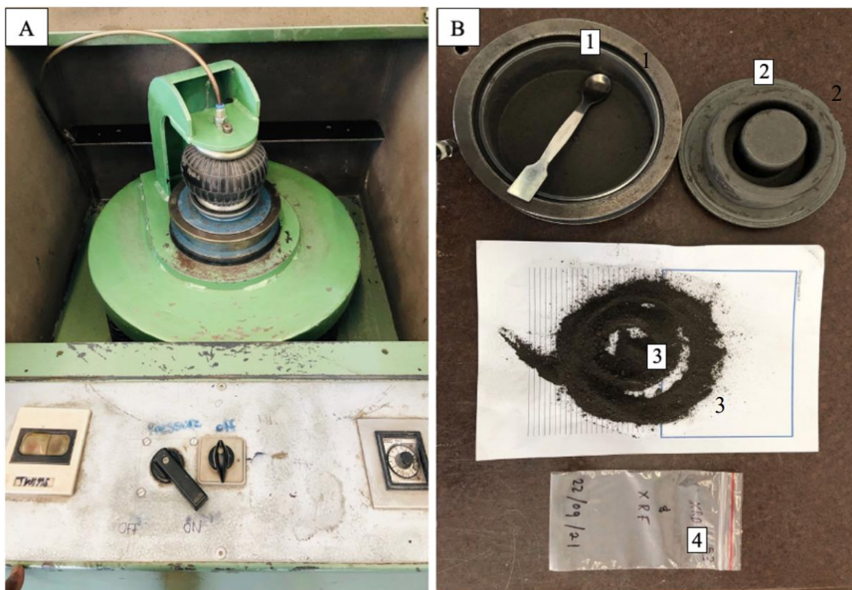
Figure 8. a) Carbon-steel swing mill used to ground the rock samples into powder for geochemical analysis. b) Photograph showing the milling dish that holds the sample material.
