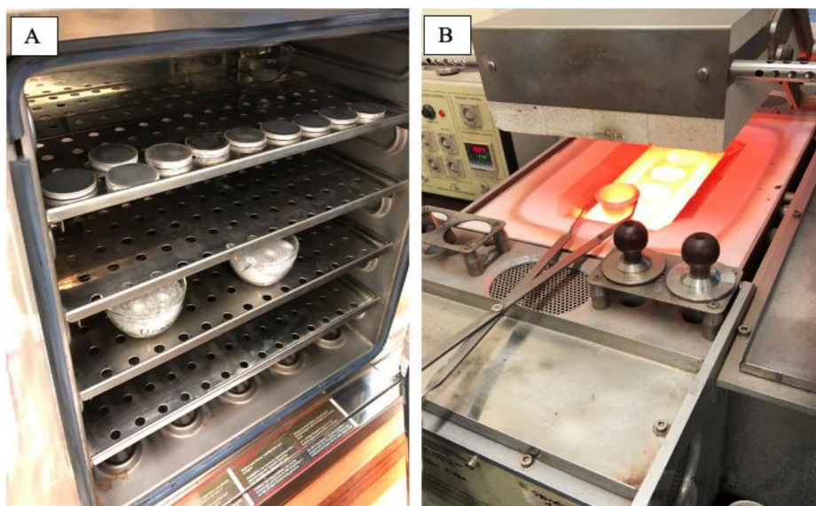
Figure 9. a) Oven used to dry the samples at various temperatures. b) Furnace used to heat XRF mixtures to 1020 °C.
