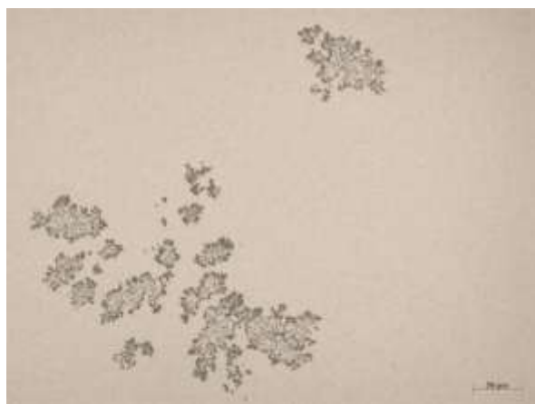
Figure A4. Eta phase in a WC-10Co (wt%) alloy – etched for 15s (courtesy of Pilot Tools (Pty) Ltd).
