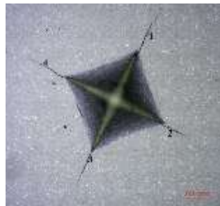
Figure 4.67. Indentation produced on 80\text{WC}-9.6\text{Co}-0.4\text{Ru} (wt%) alloy at 5 kg load with two
