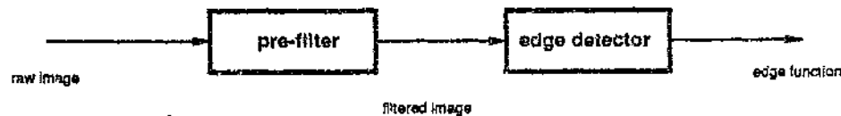
Figure 4.26: Block diagram showing a prefilter being applied to an image before edge detection in order to reduce the amount of noise resulting from differential operators.
