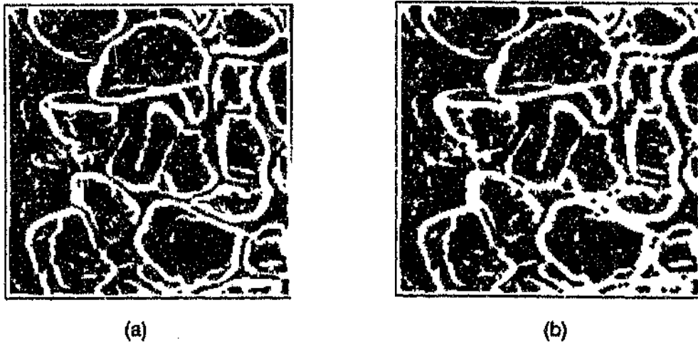
Figure 5.24: Example of closing gaps between entities in an edge image E_{p2} with a 3x3 cross structuring element (size 1) to produce fused edge images E_v . Rock is -38+25mm quartzite. (a) Edge image, (b) E_v = E_{p2} \bullet B .
