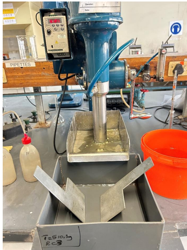
Figure 3.9: Flotation apparatus including a D12 Denver machine, 5L cell, collection tray, and scrapers.
