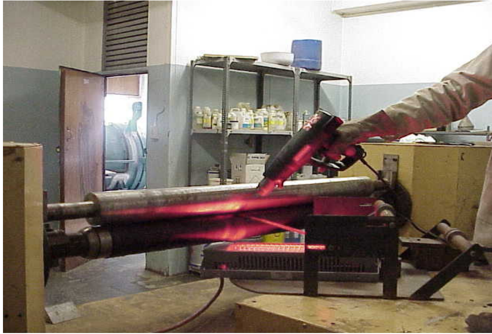
Figure 3.9: Pipe production at 35^{\circ} winding angle
