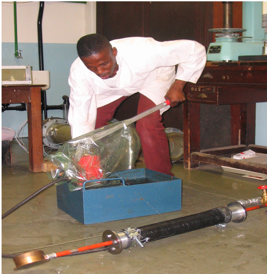
Figure 4.2: Failure of the pipe during burst test
