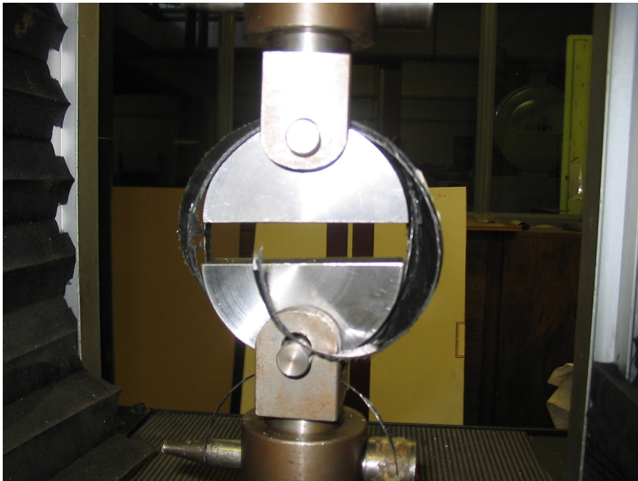
Figure 4.5: Failed test ring during the split disc test
