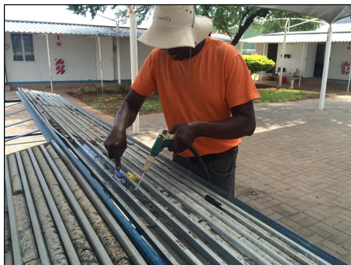
Figure 27. Core being cleaned with plastic brush to remove dust and foreign particles prior to handheld XRF analysis
