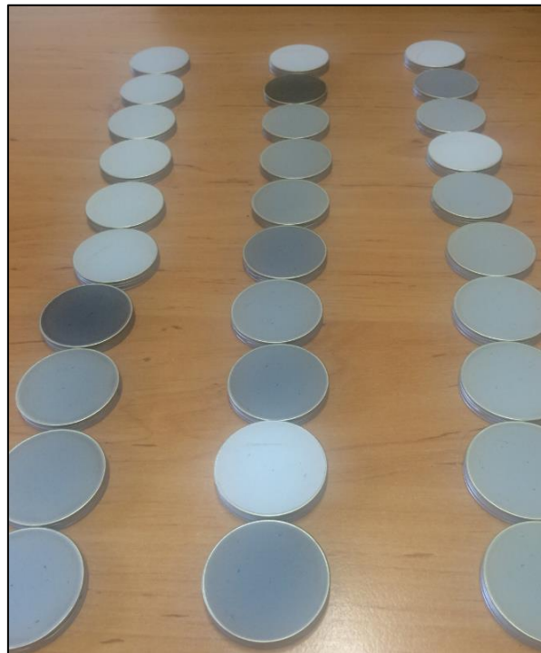
Figure 26. Laboratory prepared homogenous pressed pellets used to test accuracy and precision of handheld XRF
