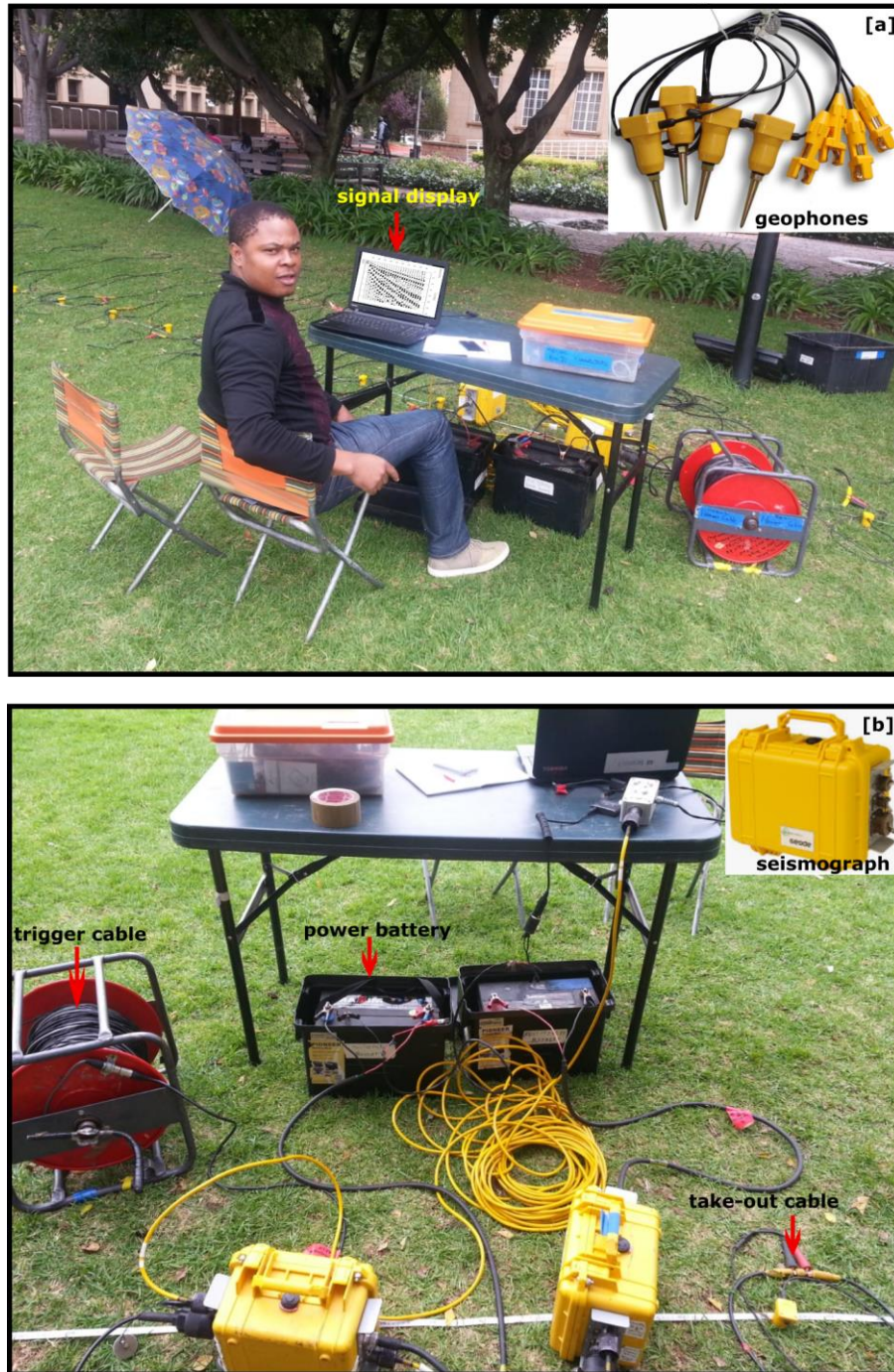
Figure 2.5: Seismic acquisition testing. (a) A laptop displaying recorded signal and geophone array, (b) is showing the Geode seismograph and trigger cable.
