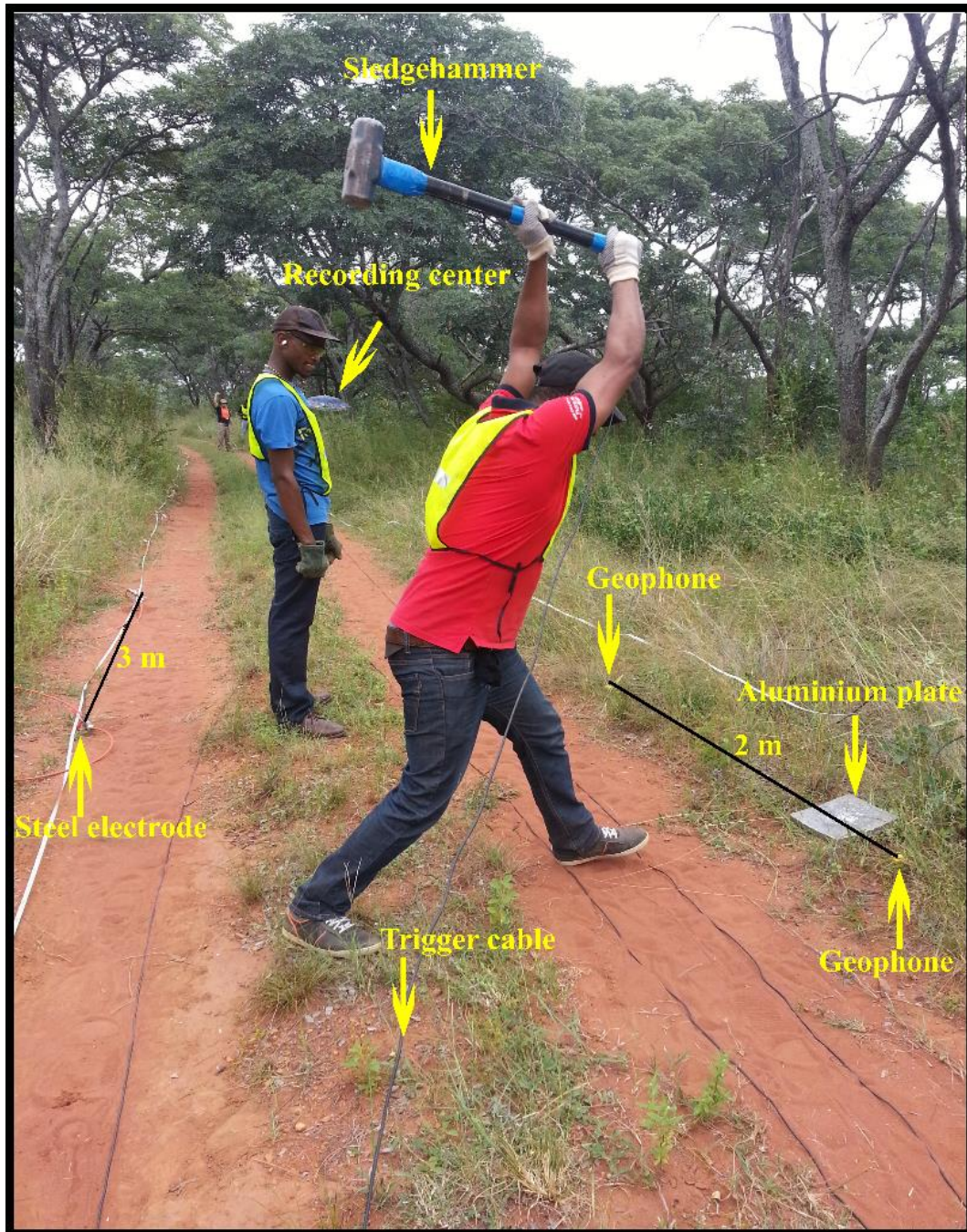
Figure 3.3: Data acquisition field setup. Line 1 is shown in the picture. On the right is 94 m seismic profile with 2 m geophone spacing; on the left, about 3 m away from seismic profile, is the 120 m resistivity profile with 3 m electrode spacing. The source is a 30 x 30 x 2.5 cm aluminum metal plate with a 9 kg sledgehammer.
