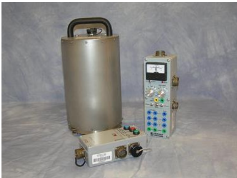
Figure 6.4: Example of seismometer used in the seismological stations.
