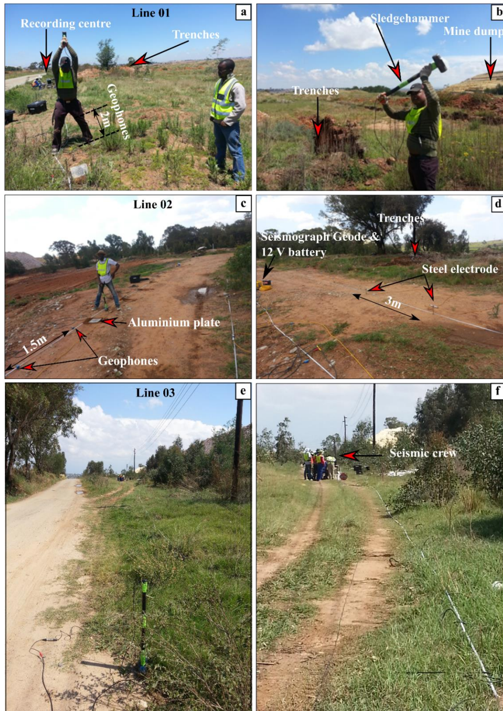
Figure 4.8: Data acquisition setup showing some mine trenches along the profiles. (a) and (b) are along L01, (c) and (d) are along L02 while (e) and (d) are along L03.
