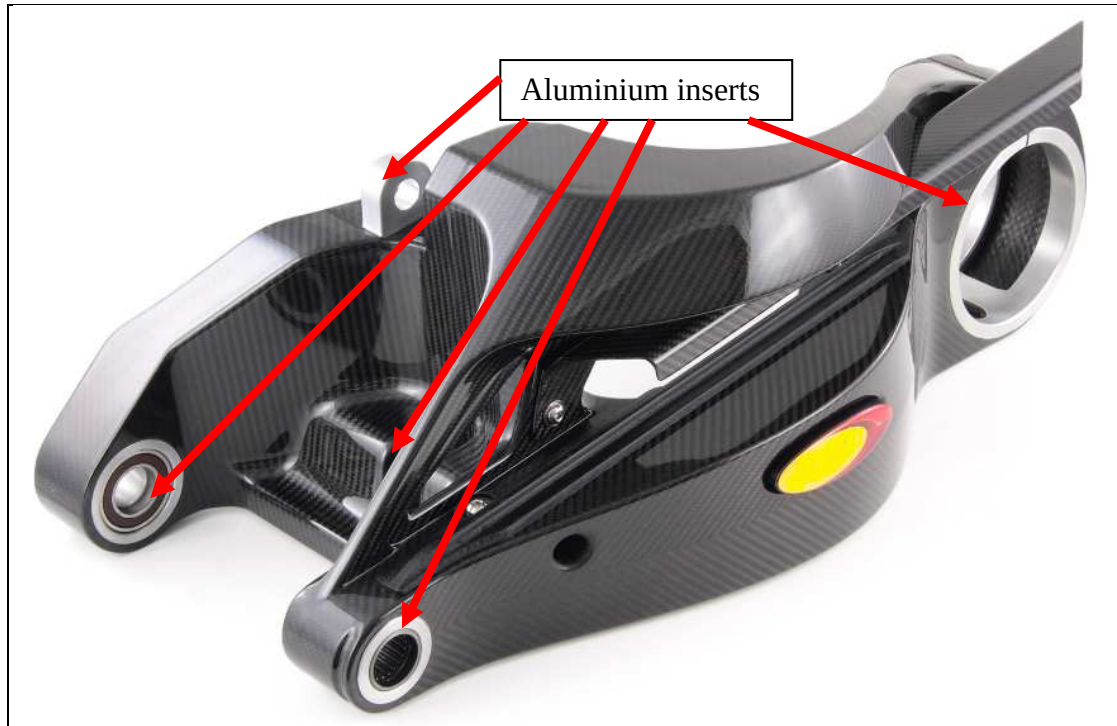
Figure 30. Swingarm showing the aluminium inserts.
