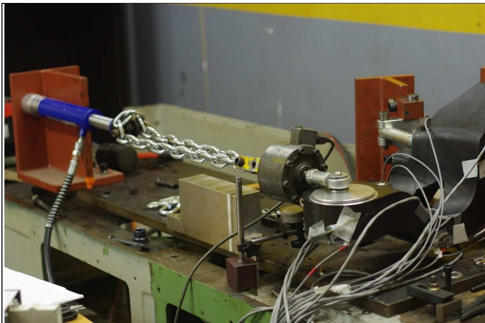
Figure 8. Swingarm test rig developed to test the carbon fibre swingarm.
