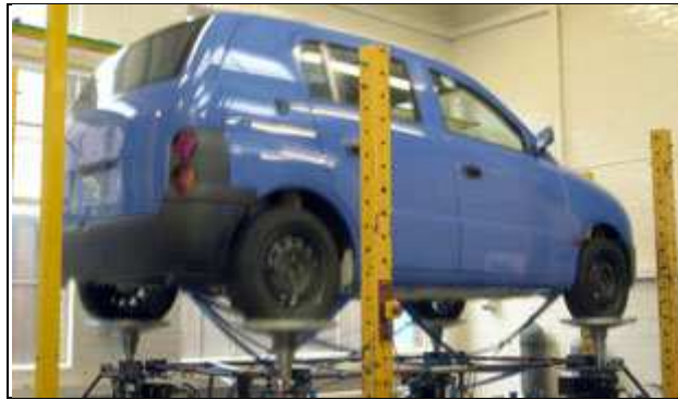
Figure 10. Durability test rig for suspension system. [25]
