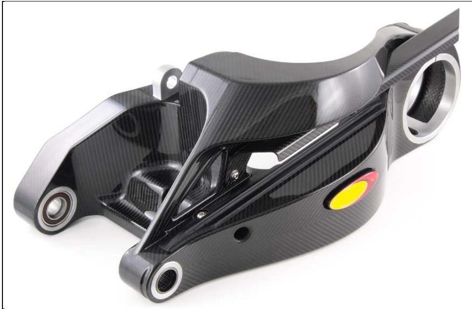
Figure 7. Single-sided carbon fibre swingarm for a Ducati 1098 motorcycle [19].
