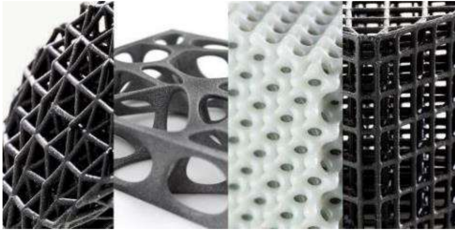
Figure 2-5. Lattice structures produced by selective laser sintering (SLS) and stereolithography (SLA) [32].
