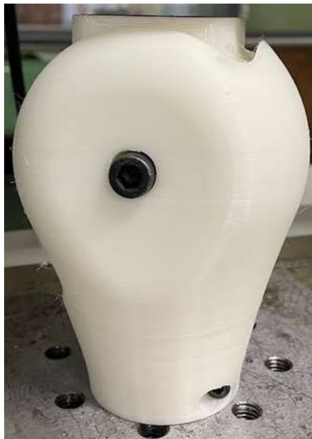
Figure 4-49. PKJ assembly after load condition I.
