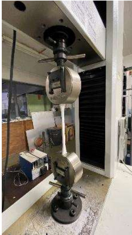
Figure 4-2. Testing of eSun eFlex TPU tensile test specimen with a UTM.
