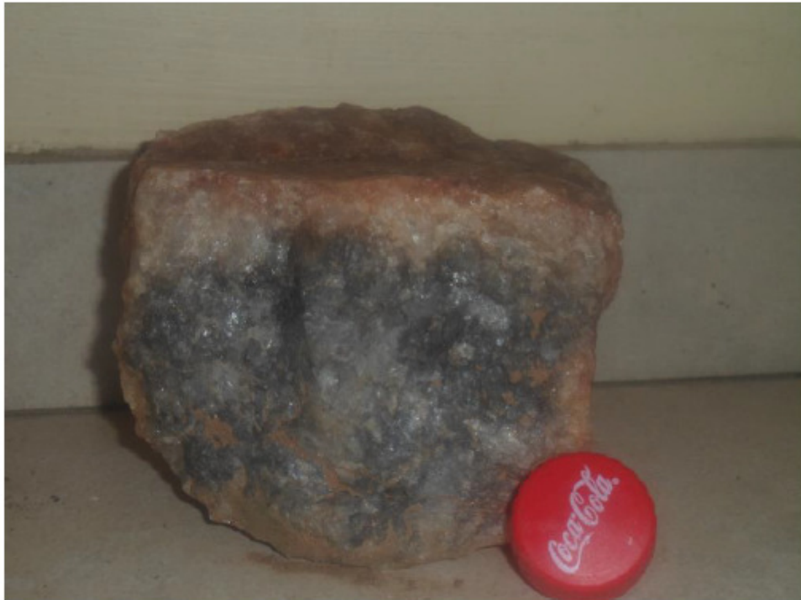
Figure 4.4: A photograph showing magnetite-quartzite at Vendome Lens
