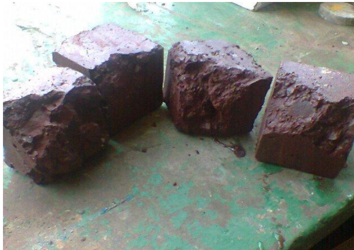
Figure 5.5: Disintegrated cubes after being placed under water
