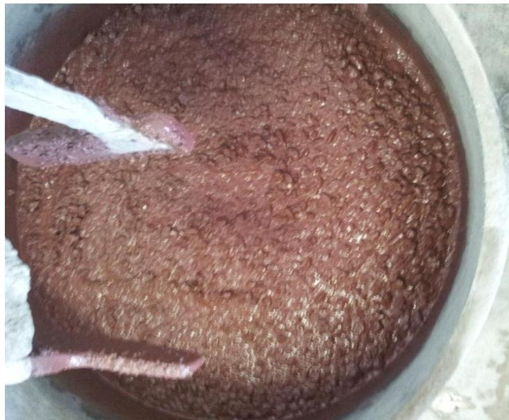
Figure 5.6: Improved fresh mixture with 3.5% and 3% dosages of superplasticiser and accelerator
