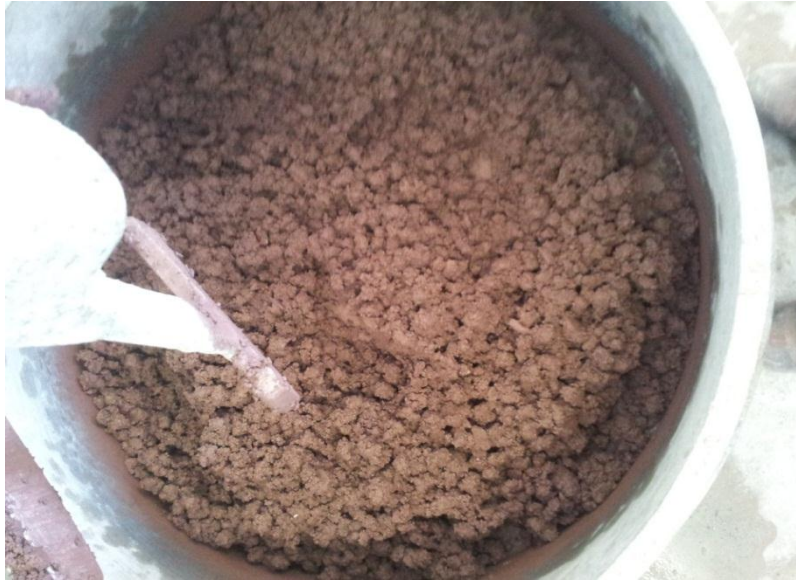
Figure 5.4: Flocculated concrete after the addition of colemanite
