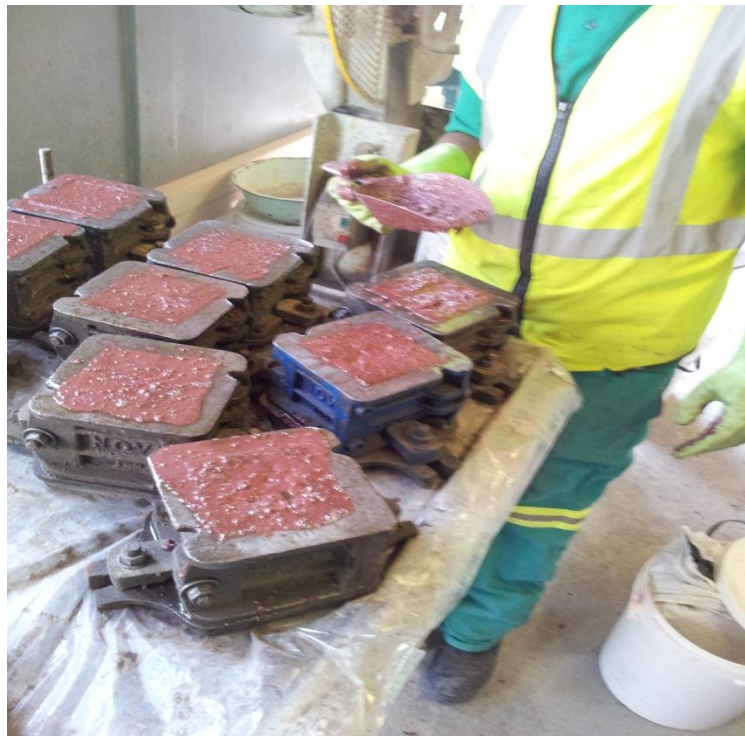
Figure 5.2: Casting of 100 x100 x 100 mm concrete cubes
