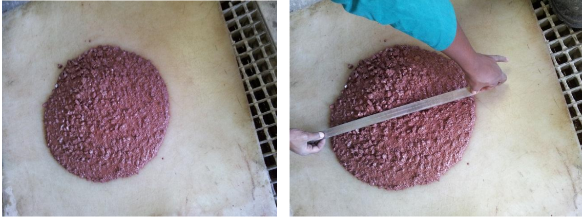
Figure 5.9: Collapsed slumps of TM6 and TM7
