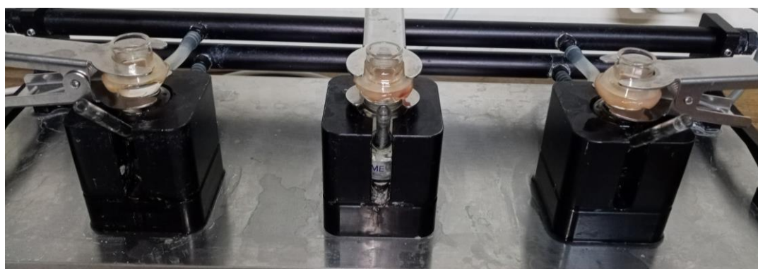
Figure 6.4: Digital image of the Franz-Diffusion apparatus setup utilised for penetration analysis.
