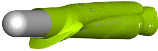
a) Viscous Simulation – Mach Number Iso-surface, M = 2.4
