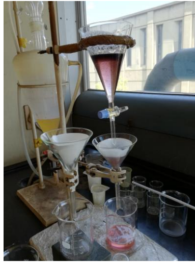
Figure 5.1: Fume cupboard set up for heavy liquid separation using Tetrabromomethane (TBE) at the Earth Laboratory in the University of the Witwatersrand.
