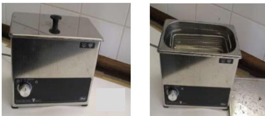
Figure 5.2 Indirect sonication system (a) closed and (b) open showing water bath
