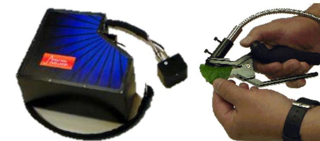
Figure 25: Spectral Evolution SR-3501 spectrodiameter machine with leaf clip apparatus for leaf level Spectral signature determination.
